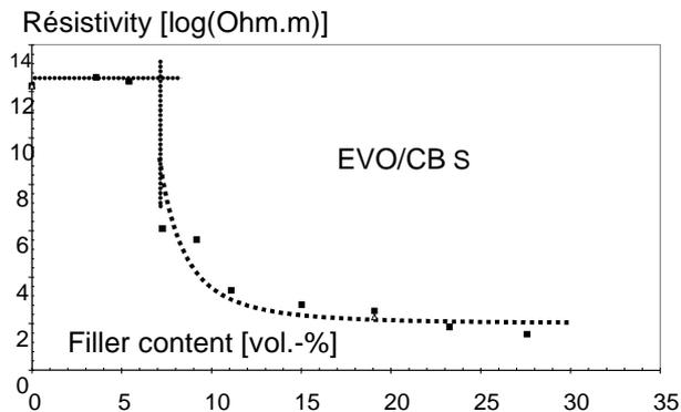
Fig. 1. Resistivity vs. CB nanoparticles concentration – percolation threshold
