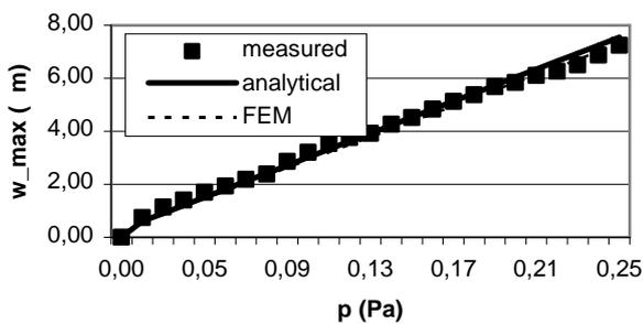
Fig. 3 Measured and estimated maximum deflection of a three-layer nanofilter membrane
