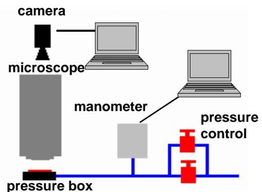
Fig. 2 Experimental set-up for breaking tests
