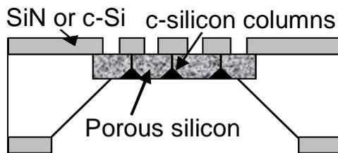
Fig. 1 Schematic view of the multi-layer membrane
