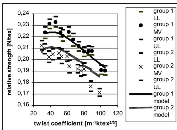
Fig. 1 Influence of twist coefficient on the polypropylene yarn relative strength (95% confidence intervals, LL-lower limit, MV-mean value, UL-upper limit)
