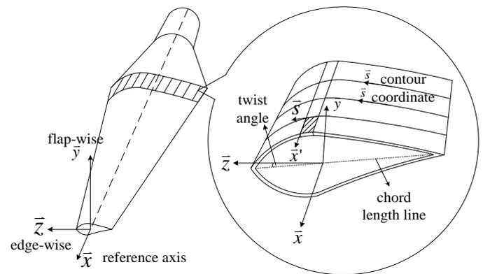
Fig. 1: Geometry, profile and the coordinate system.
