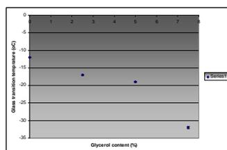
Fig. 2 Effect of increasing glycerol content on glass transition temperature
