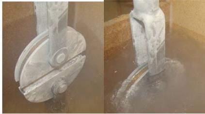
Figure 3 NOL ring tensile fixtures.
