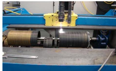
Figure 1 Laser cutting process of NOL tube.
