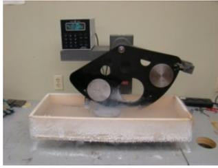
Figure 2 Test set up for NOL ring impact.
