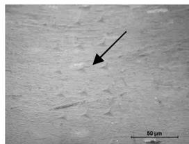
Fig.5. Indentation marks in transverse direction
