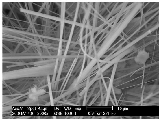
**Fig. 1** Si<sub>3</sub>N<sub>4</sub> nano-ribbons obtained by HYSYCV
