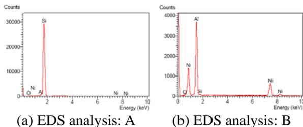
Fig. 4 Analysis of Ni/AC8A composites by SEM/EDX
