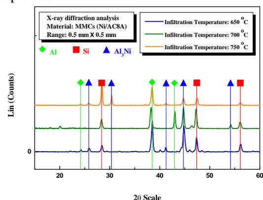
Fig. 2 Analysis of Ni/AC8A composites by XRD (X-ray diffraction).
