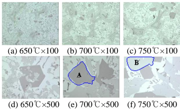
Fig. 3 Microstructure of MMC (Ni/AC8A) by optical microscope (Olympus BX60M).
