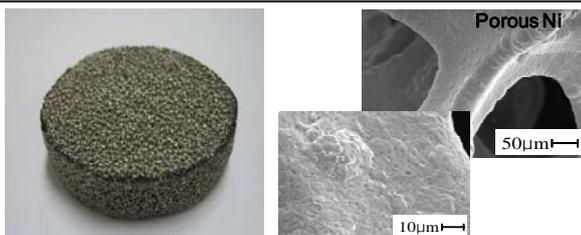
Fig. 1 Nickel porous preform for processing Metal Matrix Composite.
