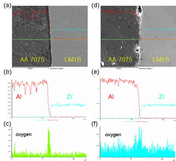
Fig. 3 Microstructure and EDS results of the co-extruded macrocomposites at region close to the interface of Samples 2 (a~c) and 6 (d-f), respectively.
