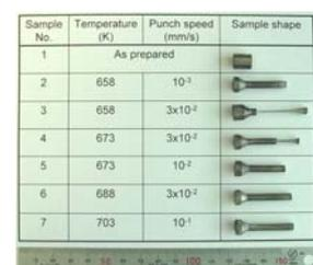
Fig. 1 LM1B/AA7075 bimetallic rods
