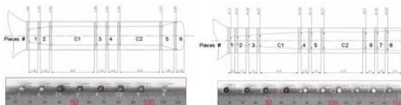
Fig. 2 Plotted images of the co-extruded bimetallic rods: (a) sample 2 and (b) sample 6.
