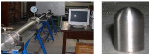
Fig. 1 high speed gas gun(Left) and impacting bullet(Right)
