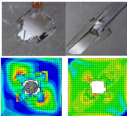
Fig. 5 Failure modes of targets at impacting velocity more than ballistic limit velocity (260 m/s); von-Mises stress result (lower right) and scalar stiffness degradation result (lower left)
