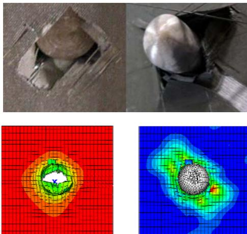
Fig. 4 Failure modes of targets at ballistic limit velocity (50 m/s); Deformation result along impacting-axis (lower left) and von-Mises stress result (lower right)
