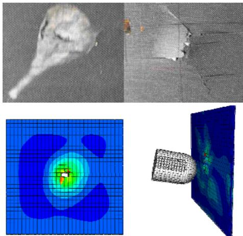
Fig. 3 Failure modes of targets at impacting velocity less than ballistic limit velocity (45 m/s); deformation result along impacting-axis (lower left) and von-Mises stress result (lower right)
