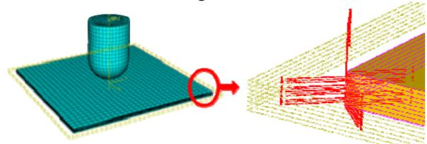
Fig. 2 Finite element model (Left) and material orientation (Right) of [(45/-45)<sub>4</sub>]s laminates
