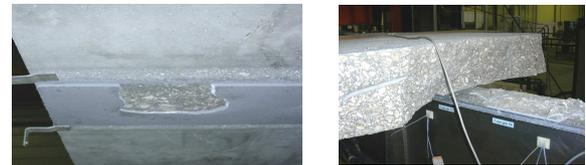
2a. Failure of the interface adhesive/steel and concrete near the steel surface
