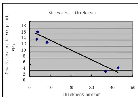
Fig 4, Relation between thickness and Maximum stress at breakpoint
