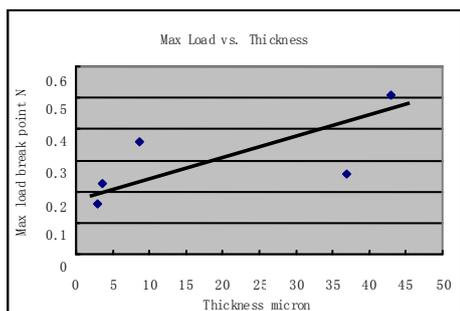
Fig 3, Relation between thickness and Maximum Load at breakpoint
