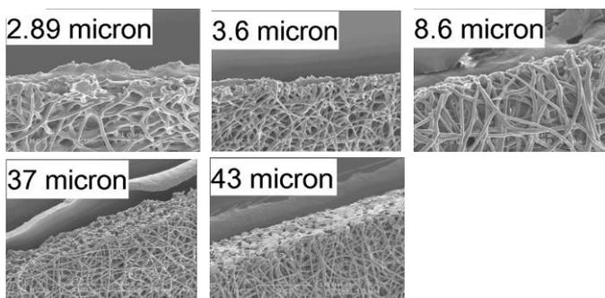
Fig 2, SEM pictures of samples with 5 different thicknesses
