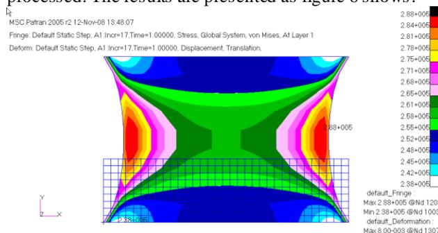
Fig 6, the globe stress of fiber section (meshed rectangle area is the original dimension of sample with thickness of 8.6 micron)
