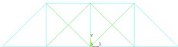
Figure 1. Schematic of a 2D truss
