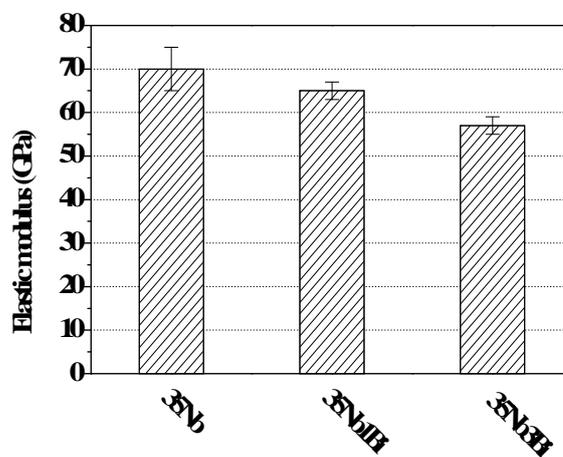
Fig. 4. Bending modulus values of Ti-35Nb, Ti-35Nb-1Bi and Ti-35Nb-3Bi alloys
