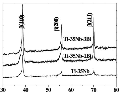
Fig. 1. XRD patterns of Ti-35Nb, Ti-35Nb-1Bi and Ti-35Nb-3Bi alloys
