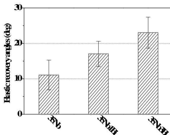
Fig. 5. Elastic recovery angles of Ti-35Nb, Ti-35Nb-1Bi and Ti-35Nb-3Bi alloys
