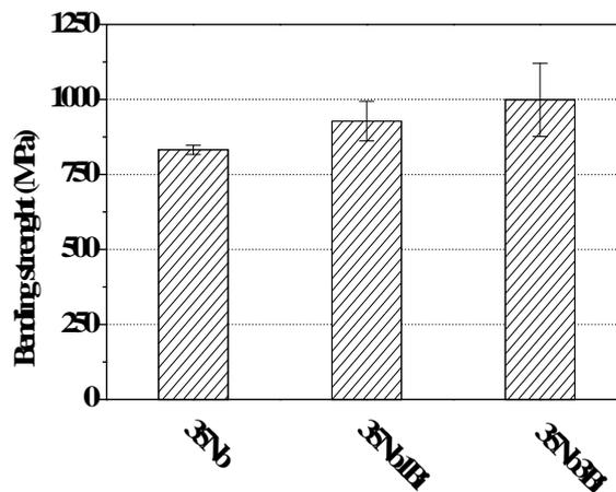
Fig. 3. Bending strength values of Ti-35Nb, Ti-35Nb-1Bi and Ti-35Nb-3Bi alloys
