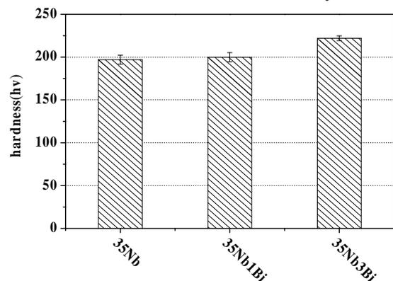
Fig. 2. Microhardness values of Ti-35Nb, Ti-35Nb-1Bi and Ti-35Nb-3Bi alloys
