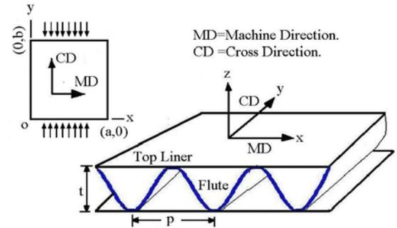
Fig. 1- Corrugated Board (CB) and the Orthotropic Plate Model.
