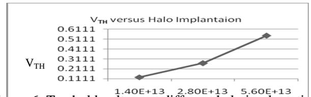
Figure 6: Threshold voltage at different halo implantation
