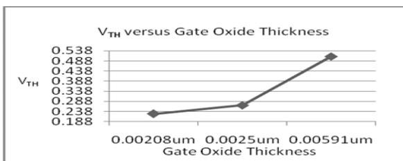
Figure 3: Threshold voltage at different gate oxide thickness
