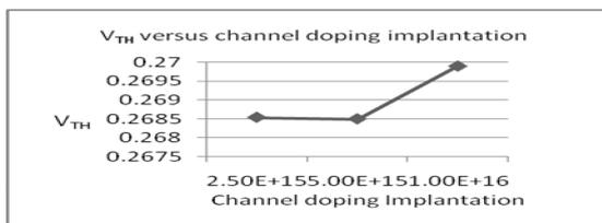
Figure 5: Threshold voltage at different channel doping
