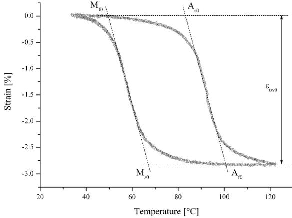
**Figure 2:** Thermally induced phase transformation in NiTi wires.
