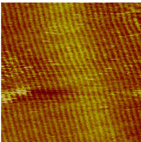
**Fig. 1 Nano-stripes formed by spin coating C<sub>20</sub>A on HOPG. The scan size of the AFM image is 150 nm.**
