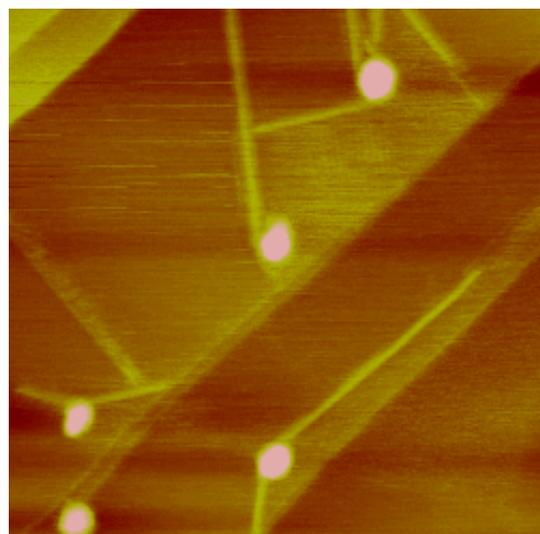
**Fig. 2 C<sub>20</sub>A nanorods nucleated on MUA-CdSe nanoparticles. The scan size of the AFM height image is 500 nm.**
