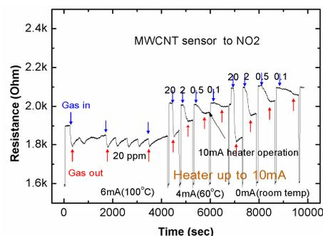
Figure 3 CNT Room Temp. response to  $\text{NO}_2$ .
