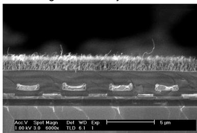
Figure 2 MWCNTs Grown on CMOS circuits
