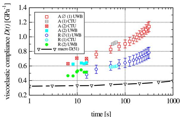
Fig.1 Comparison of creep compliance histories measured by a standard macro test ( $D(51)$ ) with average data derived from instrumented indentation tests with the loading rate 0.66 mN/s according to Eq. (1) or (2)
