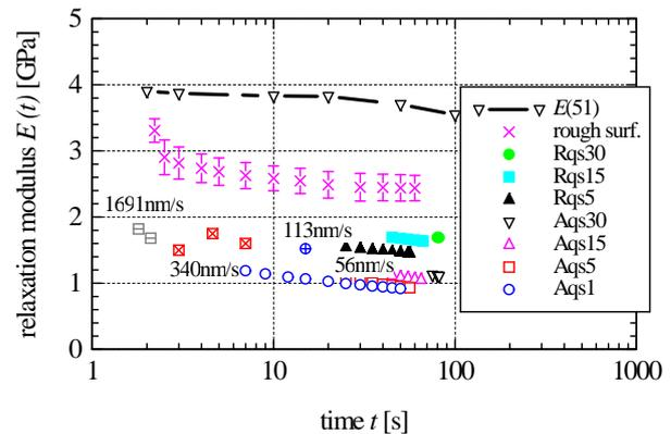
Fig. 2 Comparison of histories of the relaxation modulus measured by a standard macro test ( $E(51)$ ) with data derived from instrumented indentation tests according to Equations (3) or (4) with different rise times  $t_0$  (1s  $\leq t_0 \leq 30$ s) and different rates of penetration  $v_0$  (56nm/s  $\leq v_0 \leq 1691$ nm/s)
