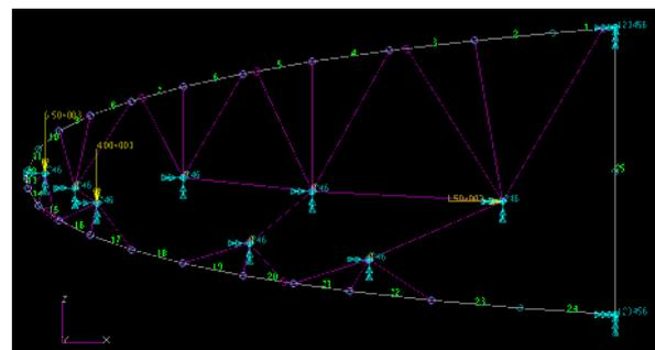
Fig.1 Actuation forces and boundary conditions
