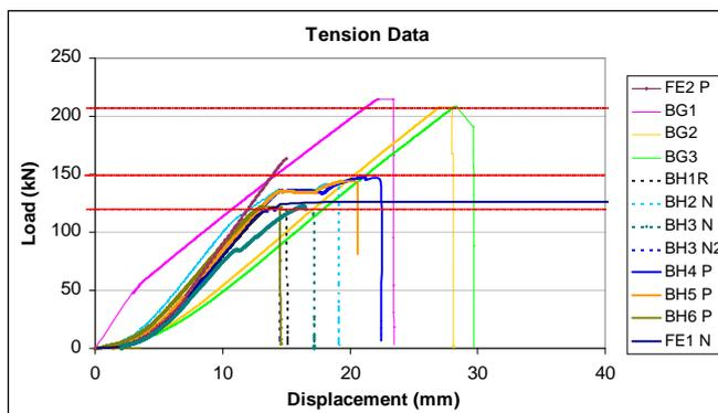
\* Note: FE1N: FE model with G8 bolt, FE2P: FE model with dowel pin
