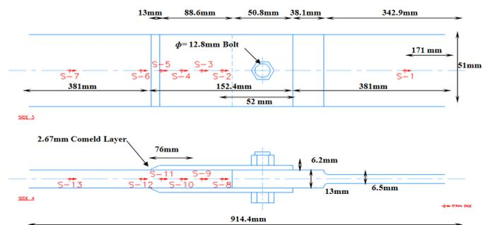
Figure 1. Hybrid joint specimen configuration.
