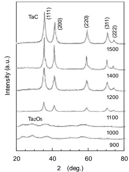
Figure 3 XRD of CA-Ta fibers pyrolyzed at various temperatures in Ar gas flow.
