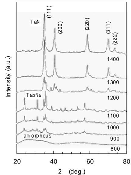
Figure 4 XRD of CA-Ta fibers pyrolyzed at various temperatures in  $\text{NH}_3$  gas flow.
