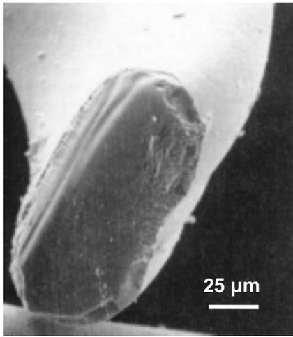
Figure 2 SEM image of CA-Ta fiber pyrolyzed under  $\text{NH}_3$  at  $1100^\circ\text{C}$ .
