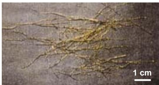
Figure 1 A view of CA-Ta fibers pyrolyzed under NH<sub>3</sub> at 1400°C.
