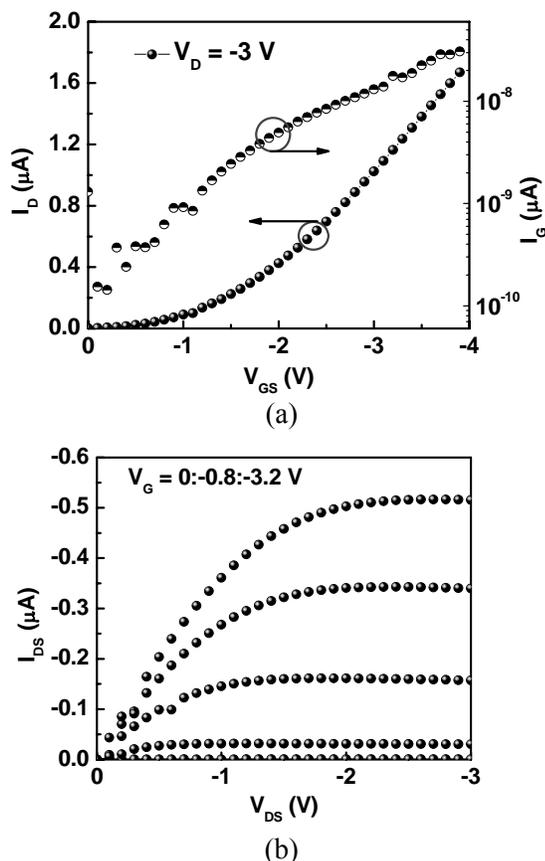
Fig. 2 Transistor characteristics (a) Drain current ( $I_D$ ) versus gate voltage ( $V_{GS}$ ) (b) Drain current ( $I_D$ ) versus drain-source voltage ( $V_{DS}$ ) of the OTFT with BDFO as the gate dielectric.
