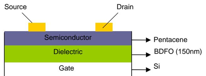
Fig. 1 Bottom-gate top-contact OTFT using BDFO as gate dielectric.
