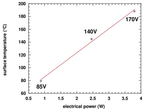
Fig. 3: Relationship between electrical power and surface temperature, as measured on a Epoxy/MWCNT composite sample for three values of the applied voltage.
