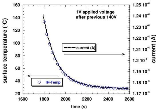
Fig. 2: Current and surface temperature, as measured on a Epoxy/MWCNT composite sample during cooling with an applied voltage of 1V, after a previous heating period, when applying 140V.
