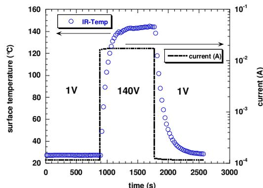
Fig. 1: Current and surface temperature, as measured on a Epoxy/MWCNT composite sample during a voltage cycle, with the successive application of 1V, 140V and again 1V.
