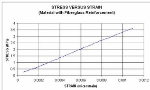
Figure 2: Stress strain curve for binder type 2
