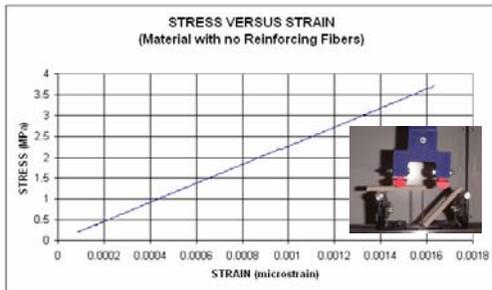
Figure 1: Example stress-strain curve for binder type 1
