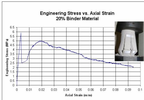
Figure 1: Representative compressive stress-strain curve
