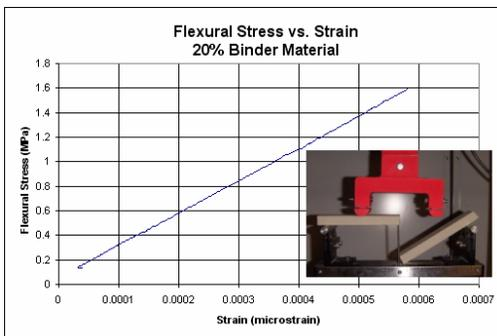
Figure 2: Representative flexural stress-strain curve
