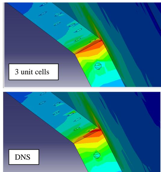
Figure 5: von-Mises stress within matrix for multi-scale model versus DNS.
