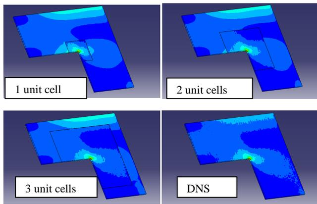
Figure 3: Results of three-dimensional simulation for multi-scale modeling method and DNS.
