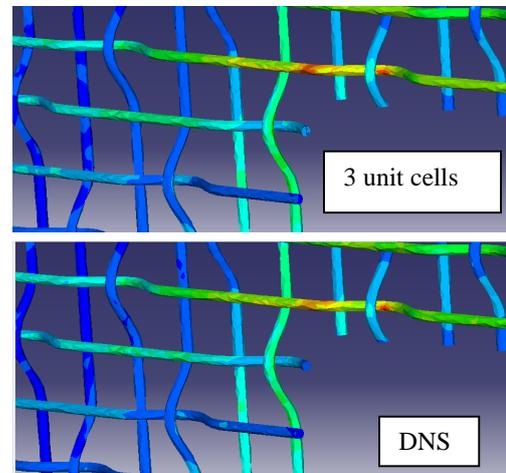
Figure 4: von-Mises stress within fiber for multi-scale model versus DNS.
