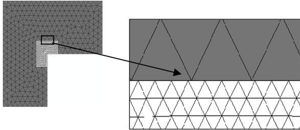
Figure 2: Averaged component mesh (gray) with embedded unit cell models (white).
