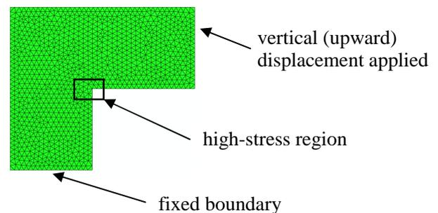
Figure 1: Geometry used for component simulation.
