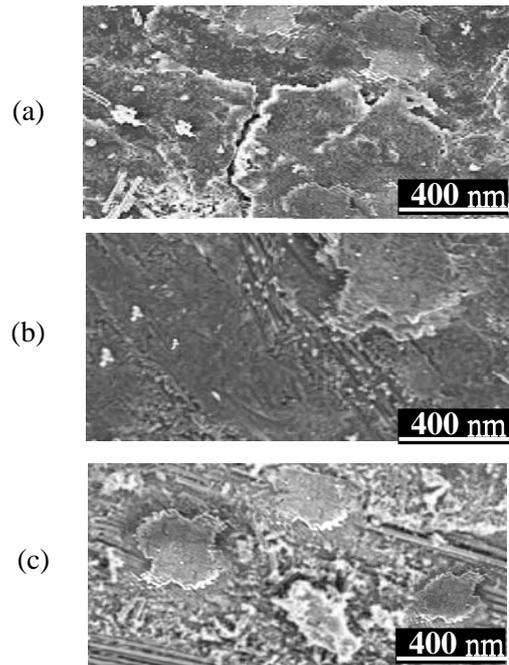
Fig.4 SEM micrograph of the worn surfaces morphological Features on PPA and its nanocomposites at high sliding speed ( $v = 3$  m/s): (a) PS10T ; (b) PS30T ; (c) PPA.
