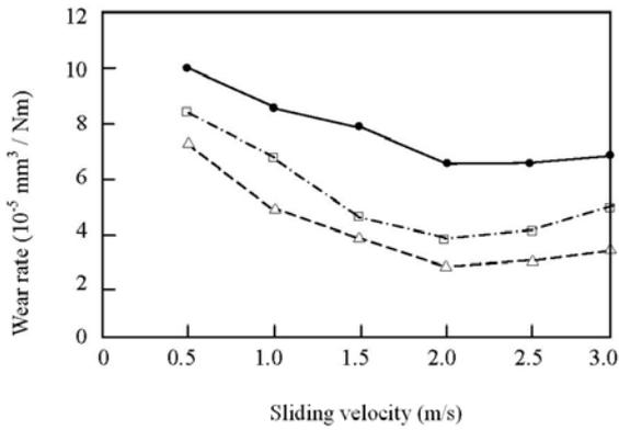
Fig. 2 Wear rate as a function of sliding velocity for pure polypropylene and silica/poly composites: (—) PPP; (---) PS30; (-.-.-) PS30T.
