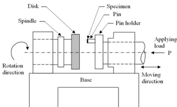
Fig.1 Schematic diagram of pin-on-disk type friction and wear tester.
