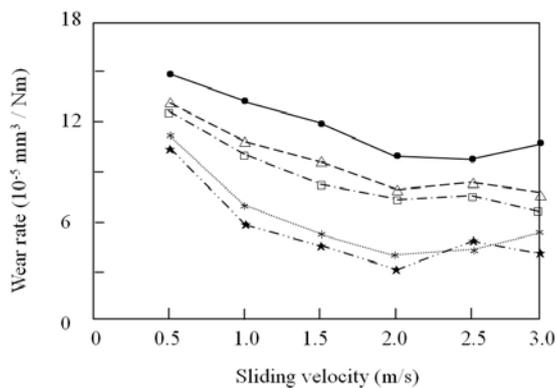
Fig. 3 Variation of wear rate with sliding velocity for PPP and silica/polypropylene polyolefin composite with various silica contents: (—) PPP; (---) PS10T; (-.-.-) PS20T; (.....) PS30T; (-.-.-) PS50T.
