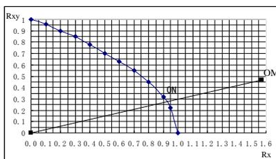
Figure1. Stiffened composite panels buckling analysis
