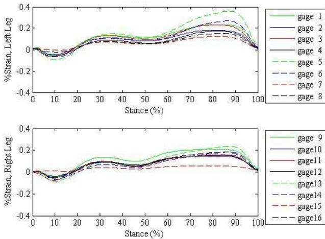
Fig 4: %Strain vs Stance (HC to TO) for CMT Subject 2
