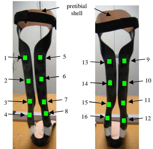
Fig 1: Gage placement on left and right HELIOS braces
