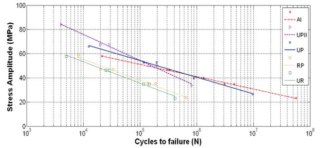
Figure 3: S-N curve for aluminium and hybrid composites laminates.
