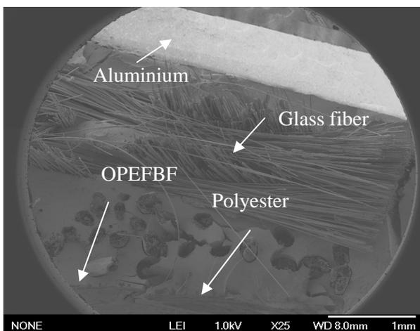
Figure 9. Scanning electron micrograph of tensile fractured surface of alkali treated hybrid aluminium composite laminates. (magnification X 37)
