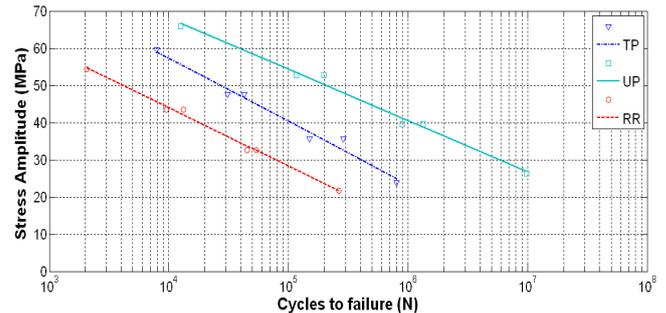
Figure 4: S-N curve for UP, TP, and RR hybrid composites laminates.
