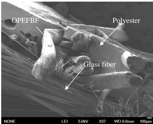
Figure 8. Scanning electron micrograph of tensile fractured surface of untreated hybrid aluminium composite laminates. (magnification X37)
