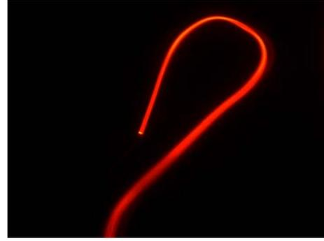
Fig. 2 Fluorescence image of fiber made by a red-emitting polymer. Fiber diameter  $\cong 1$   $\mu\text{m}$ .
