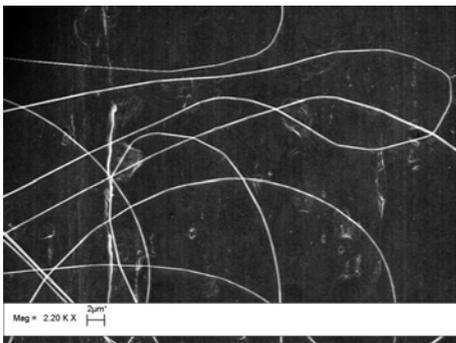
Fig. 1 SEM micrograph of infrared light-emitting nanofibers, as collected after electrospinning.
