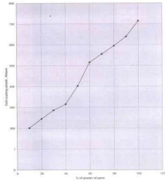
Fig4 :CSS OF FLY ASH PLASTER OF PARIS COMPOSITE
