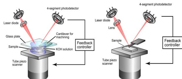
Fig. 1 Schematic diagram of experimental method for simple nanoscale scratching (left) and hybrid nano-fabrication.
