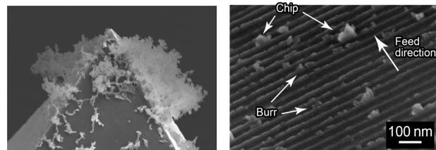
**Fig. 3** SEM image of pyramidal diamond tip after machining a silicon substrate(left) and machined silicon surface(right).
