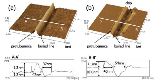
**Fig. 2** Enlarged AFM topography image of single line fabricated (a) using a blunt tip. (b) using a sharp tip.
