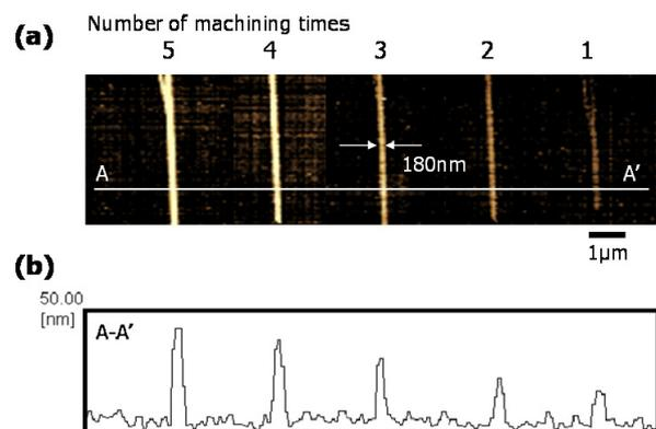
**Fig. 4** (a) An array of silicon bars prepared according to hybrid nanofabrication (b) Cross-sectional topography trace of a line marked A-A' in (A).
