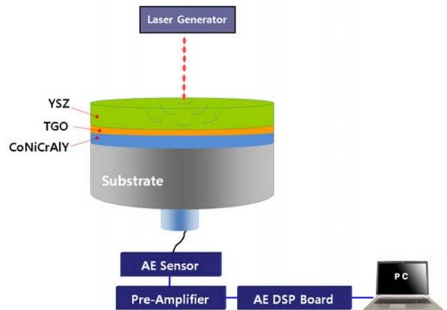
Fig. 1 Schematic diagram of laser and AE system
