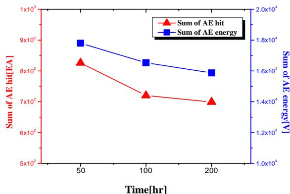
Fig. 3 AE hit and energy depending on thermal oxidation time
