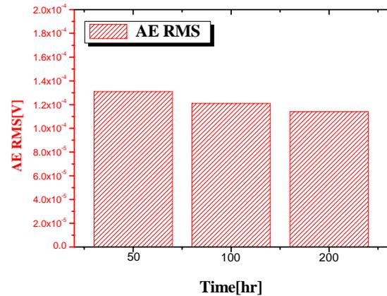
Fig. 4 AE RMS depending on thermal oxidation time
