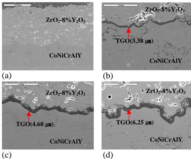
Fig. 2 SEM images of cross section after thermal oxidation test (a) as-sprayed (b) 50hr (c) 100hr (d) 200hr
