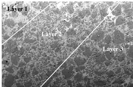
**Fig. 1** Optical photomicrograph of a three-layer composite.
