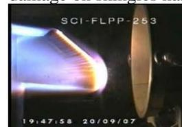
Figure 7- CMC demonstrator under plasma testing (SPS, CIRA, VKI)
