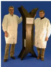
Figure 4- Thrust frame for two gimballed engines (2 x 87.2 kN) (SABCA-SONACA)
