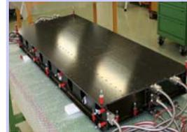
Figure 6- Fiber Optic, Health Monitored, Heat Resistant CFRP Airframe Structure (RUAG)
