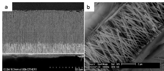
Fig.1 (a) SEM images of the Au nanowires showing partial deposition of Au nanowires in AAO membrane and (b) full length of the membrane in polycarbonate membrane for 30 min deposition time
