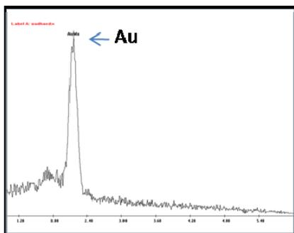
Fig.3 The elemental composition of Au nanowires were measured by EDAX
