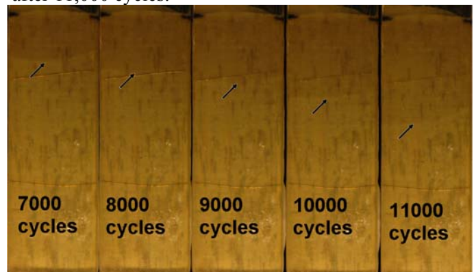
Figure 6. Photographs of disbond growth from the end of the GFRP adherend (which is also the low wavelength end of the CFBG)
