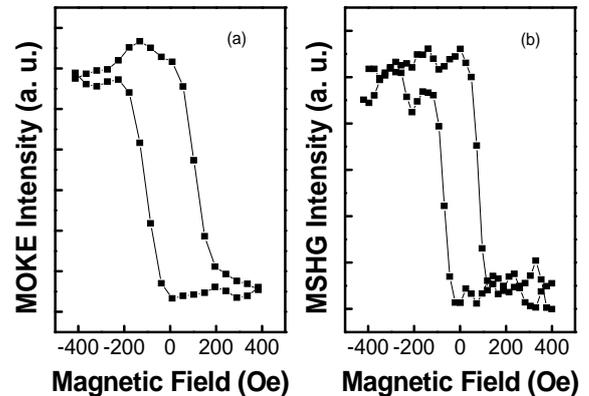
Fig. 2 MSHG and MOKE hysteresis curves: MSHG intensity for *Fe/Al* film measured in longitudinal geometry, with p-polarized incidence and an analyzer angle of 45 degrees relative to s-polarization. (a) shows MOKE loop: 25-nm *Fe* film with a cap layer of *Al* (5-nm). (b) shows its relative MSHG loops.
