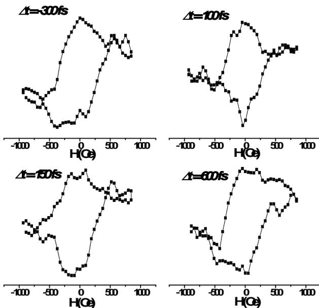
Fig. 3 Time-resolved Faraday rotation on 50-nm Fe magnetic nanoparticle arrays with a cap layer of Pt (5-nm).
