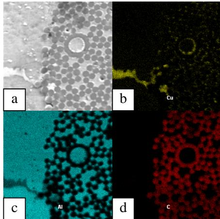
Fig. 2: SEM, and EDS Dot mapping of A206-CFW composite. a) SEM microstructure of transverse section of fibers b) Cu dot map, c) Al dot map, d) C dot map.
