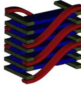
Fig. 1: 3D CFW showing weave nomenclature; Stuffers shown in blue = Warp fibers, X-direction; Filler shown in green = Fill fibers, Y-direction; Warp Weaver shown in red = Z-direction
