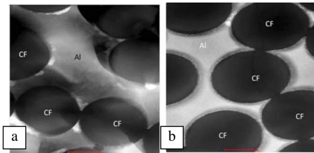
Fig. 4: TEM images (fiber diameter approximately 5 microns) of the A206-CFW composite. a) As-cast, b) T7 heat treated.
