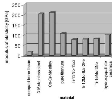
Figure 1: Modulus of elasticity values for typical and new generation metallic alloys used for implant manufacturing.
