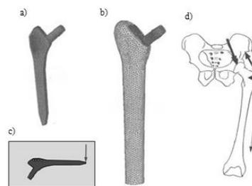
Figure 2: Model of implant (a), model of implant – bone complex (b), model of load used in stiffness characteristic calculations (c) and model of loading used in shear strain distribution analysis (d) .
