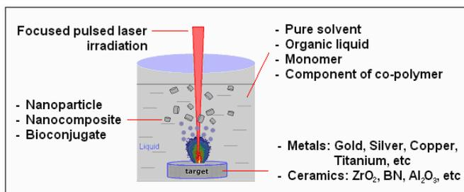
Fig. 1 General routes to rapid nanocomposite manufacturing by laser ablation in liquids
