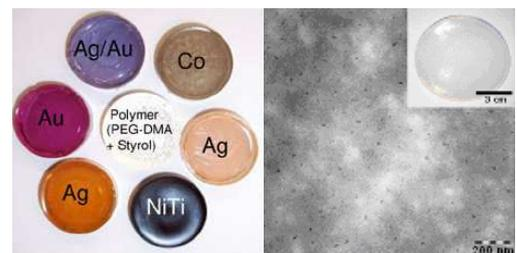
Fig 2 (Left) Examples of manufactured nanocomposites with embedded metallic nanoparticles. (Right) TEM image of gold nanoparticles embedded into acrylic polymer.
