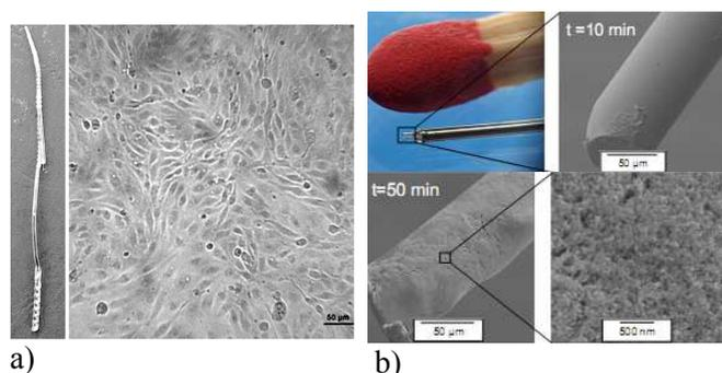
Fig. 3 (a) Silicone electrode mantle of a cochlear implant and Endothelial cells grown on a silicone-silver nanoparticle composite. (b) Pt/Ir neural electrodes coated with fs-laser generated platinum iridium nanoparticles for improvement of neural contact using electrodeposition [3].
