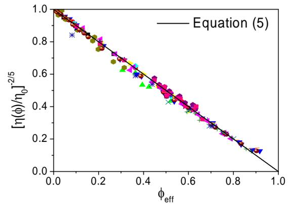
Fig.1: Master curve for the viscosity as a function of  $\phi_{eff}$  for hard-sphere suspensions. Symbols represent experiments and the solid line our theory, Eq. (5).
