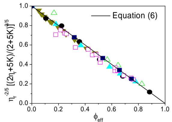
Fig.2: Master curve for the viscosity as a function of  $\phi_{eff}$  for emulsions. Symbols represent experiments and the solid line our theory, Eq. (6).
