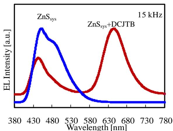
**Fig. 2** Frequency dependence of the emission spectrum of red-emitting organic-dye-dispersed powder EL device.
