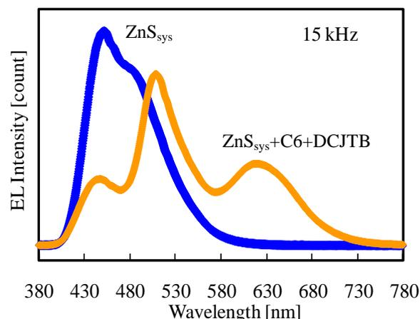
**Fig. 3** Frequency dependence of the emission spectrum of white-light-emitting organic-dye-dispersed powder EL device.
