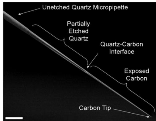
Figure 1: SEM micrograph of a CNP tip. Scale bar, 5  $\mu\text{m}$ .
