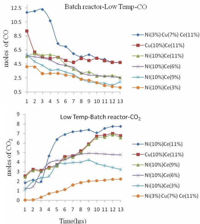
Figure 5: Gas phase batch reactor CO conversion and CO<sub>2</sub> production data of LTS catalysts
