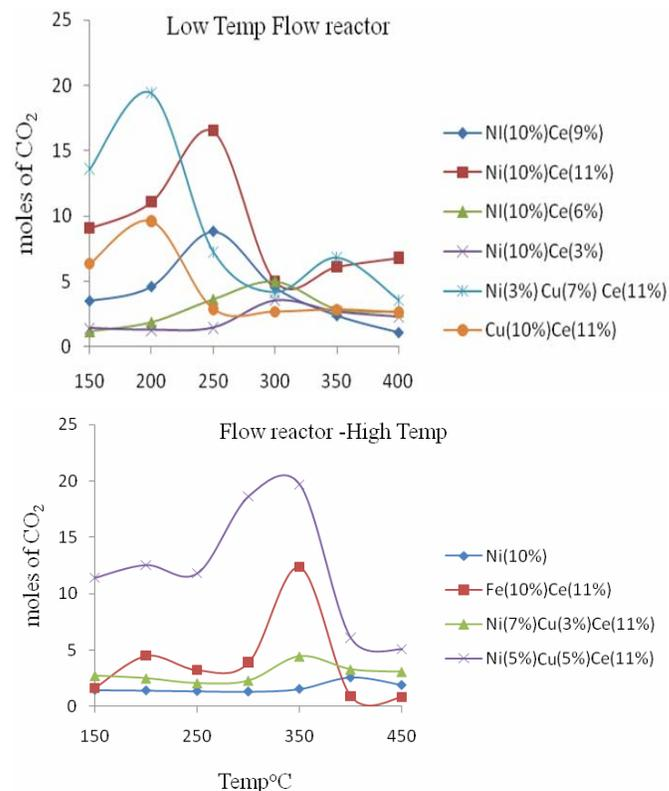
Figure 4: Comparison of gas phase dynamic flow reactor data of LTS and HTS catalysts
