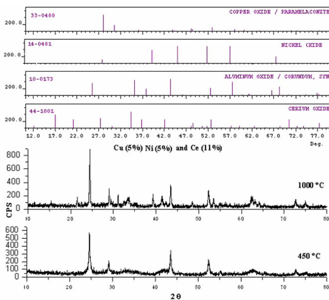
Figure 3: PXRD spectra at 450 °C and 1000 °C for Cu(5%)Ni(5%)Ce(11%)/alumina
