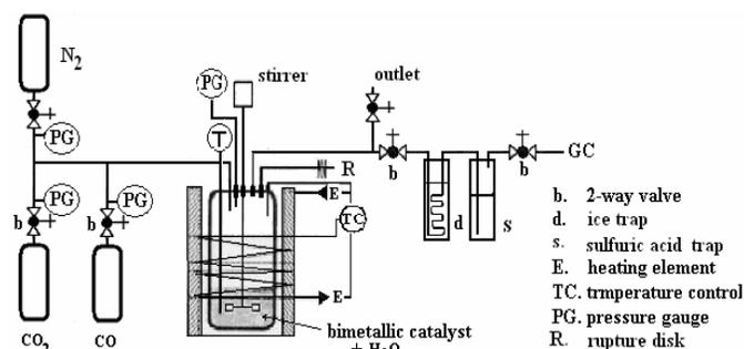
Figure 2: Gas-phase batch reactor for kinetic study of WGS catalysts
