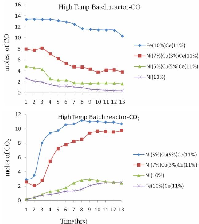
Figure 6: Gas phase batch reactor CO conversion and CO<sub>2</sub> production data of HTS catalysts
