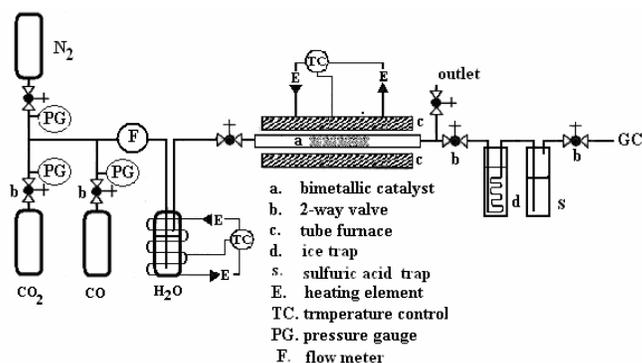
Figure 1: Gas-phase flow reactor for optimizing WGS reaction parameters
