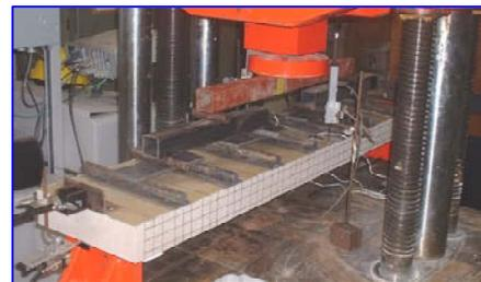
Figure 1 Experimental setup of uniformly loaded panels
