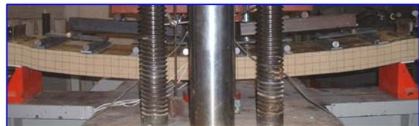
Figure 5 Deflected shape of sandwich panels
